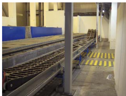
Alle Niederlegungen in Schutzblech verriegelt (IPROJADET) Mindesthöhe = 330mm All rails lines are passed through a fire protective base (IPROJADET) with thickness = 330mm
